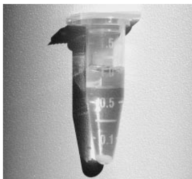
Figure 4. Photograph of precipitate resulting from centrifugation of a 1% AcOH solution of crude peptide P3 synthesized manually using capping reagent 2 . The supernatant contains largely the full-length peptide. Similar treatment of the Ac 2 O capped crude peptide mixture does not result in any observable precipitate.
